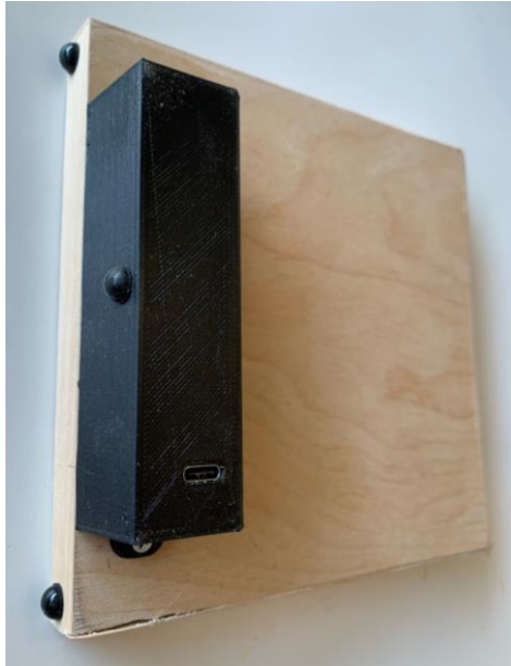
Figure 11. Enclosure attached to back of CLOQ and rubber feet installed
