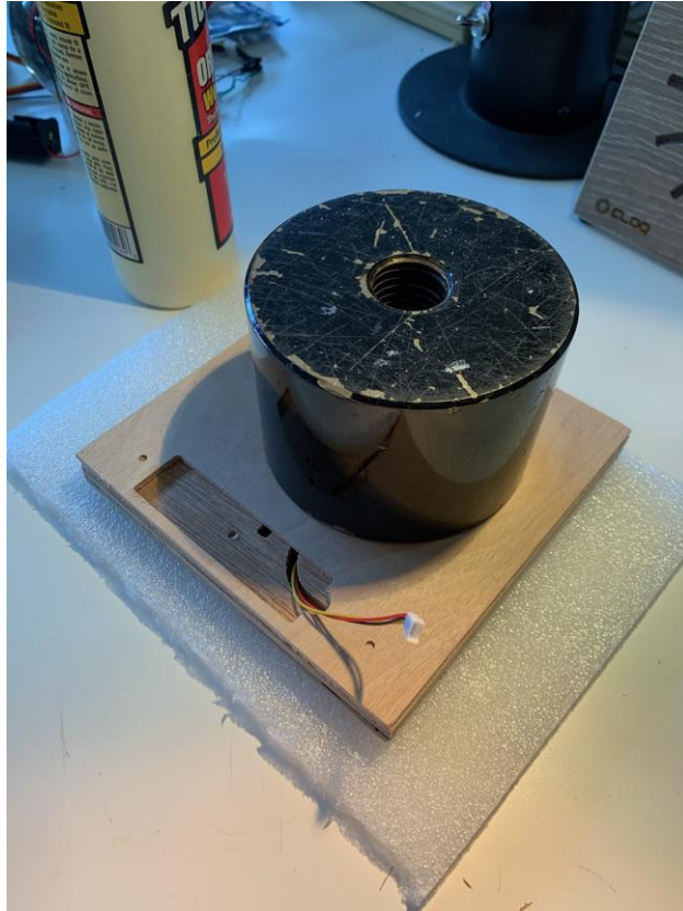
Figure 5. Align and attach CLOQ back. Weight is placed while glue is drying.
